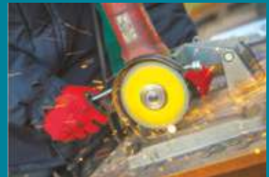
Cutting test – a test for wheel durability
