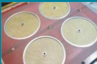
Placing of the second reinforcing element
