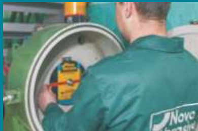
Safety test – wheel bursting speed test
